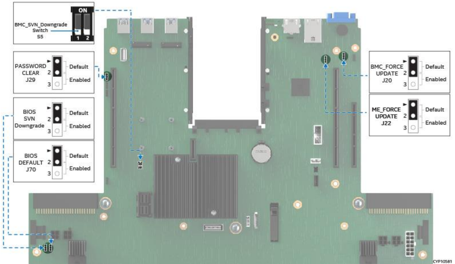
Figure 7. System Configuration and Recovery Jumpers
