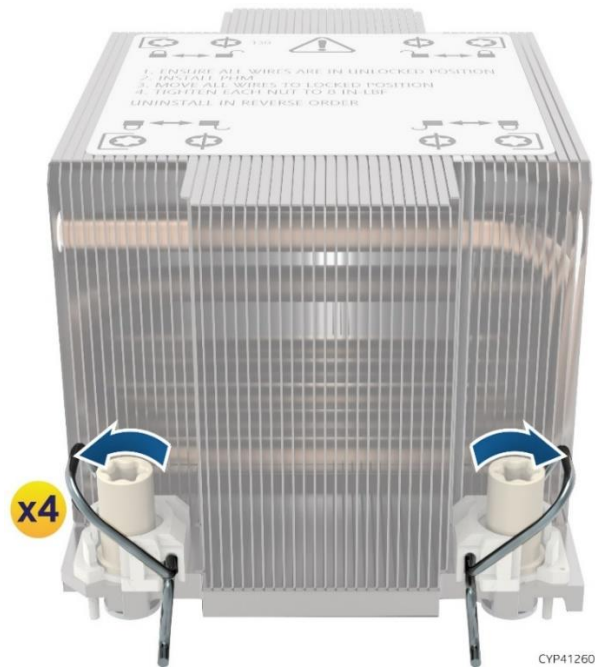
Figure 78. Processor Heat Sink Anti-tilt Wires in the Outward Position
